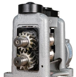
You can now grease the gears
