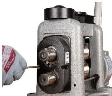
Remove 2 screws and cover
